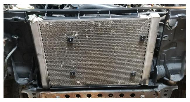
Apply 1 strip of the supplied Foam with adhesive backing, to both top and bottom of the radiator.
