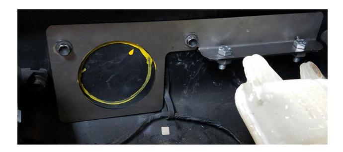
You will then need to cut off the intake tube from your air filter housing. You will weld the supplied Cap over the void in the filter housing. Use the portion of the intake tube you just removed, and weld it inline with the new fender inlet.
